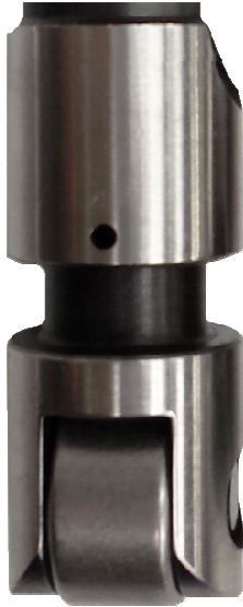
Figure 1: Stock un-modified solid roller lifters
